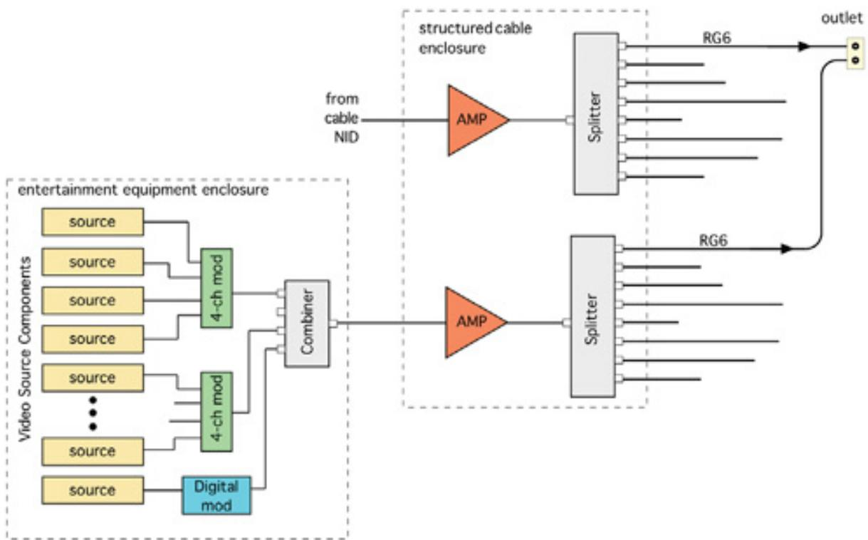
An alternate dual-cable architecture avoids the channel-sharing problem by separating the downstream channels into two physical cables.
