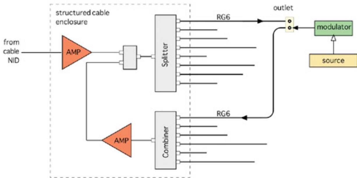
The typical dual-cable architecture became popular in the mid-90s as a way of providing an internal cable path back to the structured enclosure. Difficulties have risen, however, as unused cable channels on which to place modulated signals are rarer.
