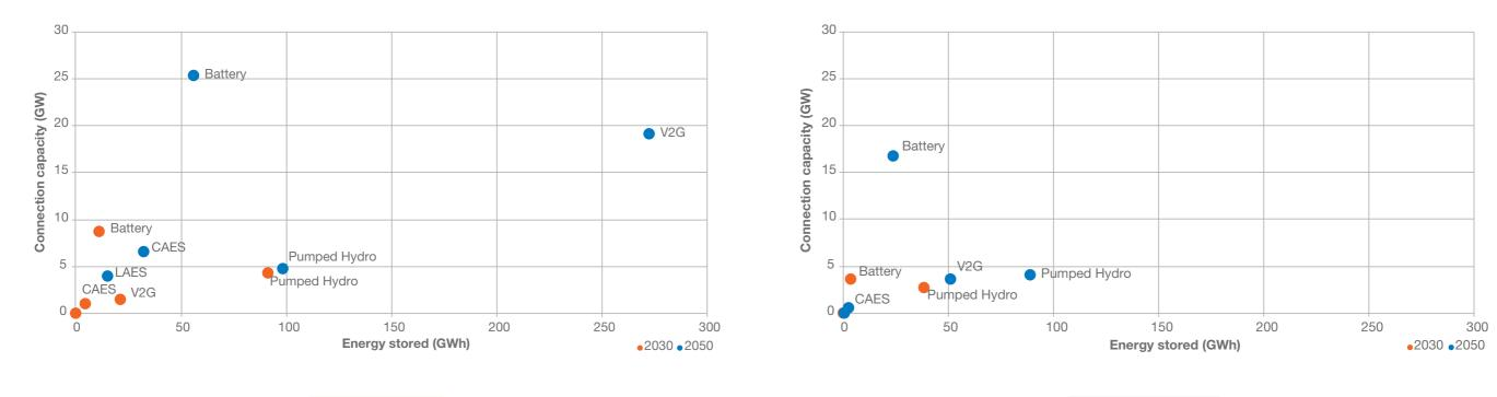
Figure SV.45: Varying power and energy outputs of electricity storage types in 2030 and 2050<sup>3</sup>
