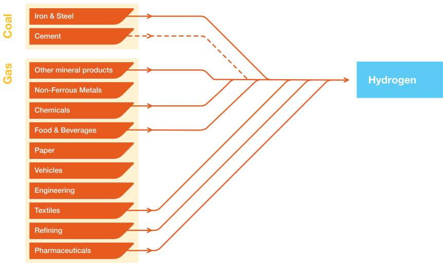
Figure CV.7: Industrial fuel switching options for decarbonisation
