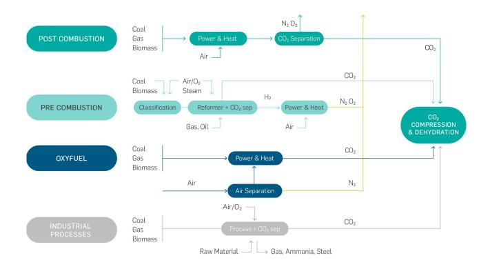
FIGURE 21 CARBON CAPTURE AND STORAGE PROCESS [REF. 101]
