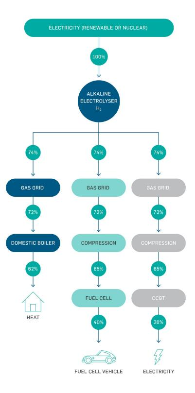
FIGURE 20 HYDROGEN PROCESS EFFICIENCY
