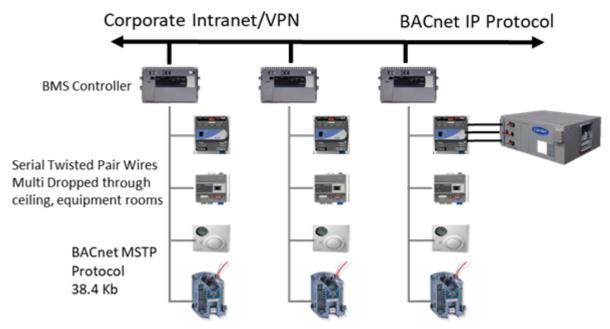
Figure 1 – Typical Sensor Network Connection
