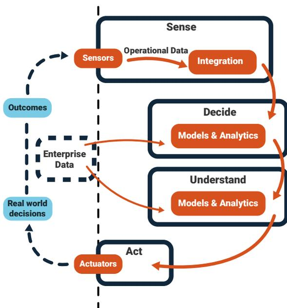
Figure 2: Digital twin conceptual architecture
